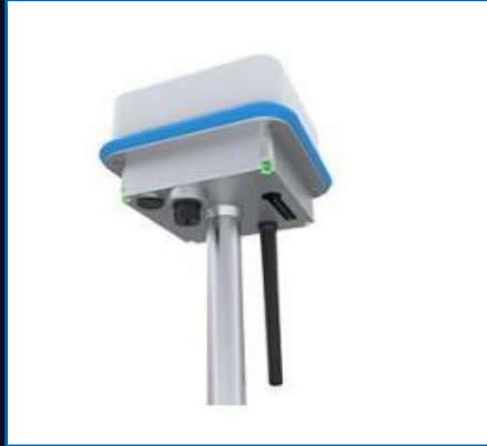
RTK Mobile Base Station
